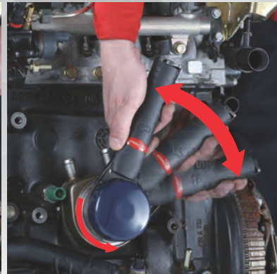
Ratchet effect ensures quick tightening and loosening
