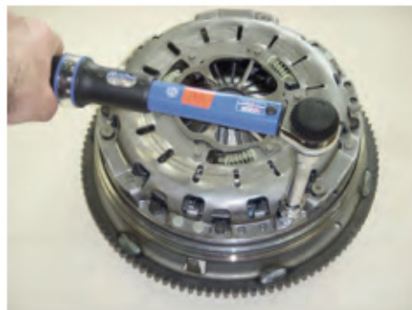
17. Screw the missing cover fastening screws into the now free threaded receptacles on the flywheel hand-tight. At the end, tighten all fastening screws with the torque stipulated according to the manufacturer's specifications.
