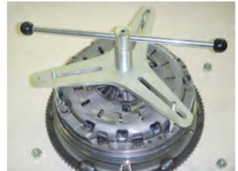
15. Loosen hexagonal nuts - remove clamping device.
