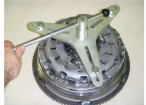
12. Screw the pressure spindle onto the catch until the disc spring is actuated. Attention: Only turn until the cover of the pressure plate touches the support of the disc flywheel.
