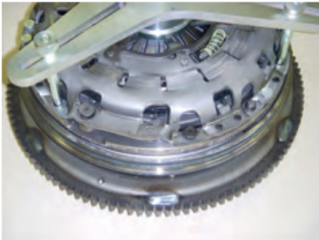
13. Tension disc springs.
