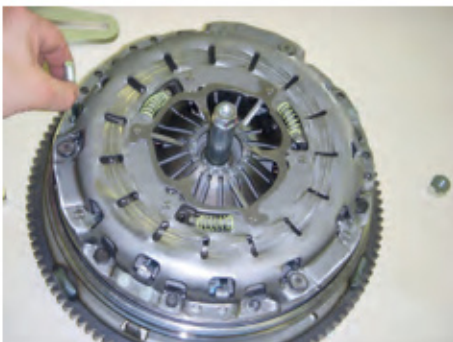
16. Remove threaded bolts.
