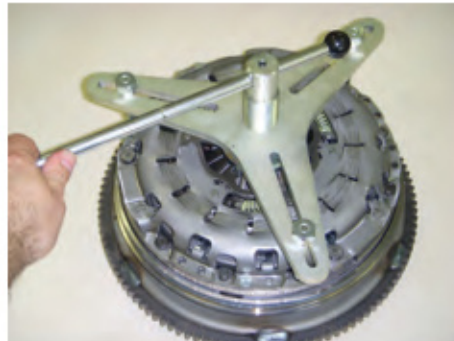
14. Completely turn back the pressure spindle - disc spring will release tension.
